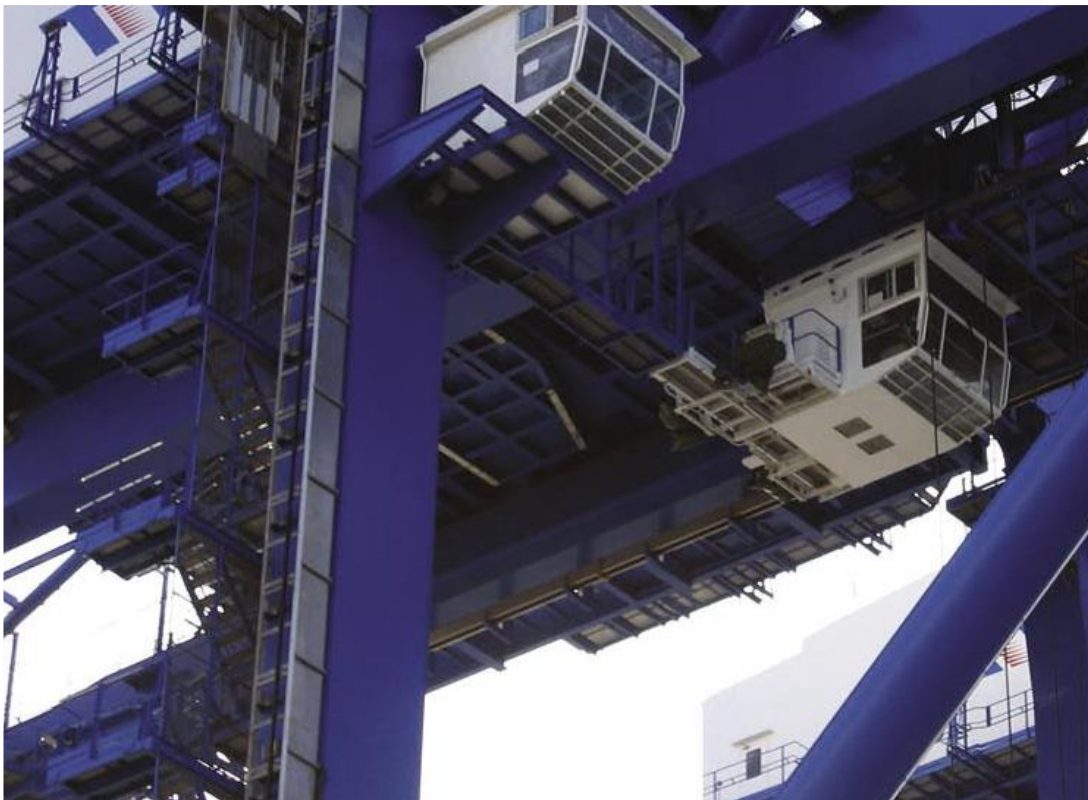
Figura 8: Grúa con cabina de control fija ( https://new.siemens.com/global/en/markets/cranes/harbor-cranes/final-landing-system.html )
